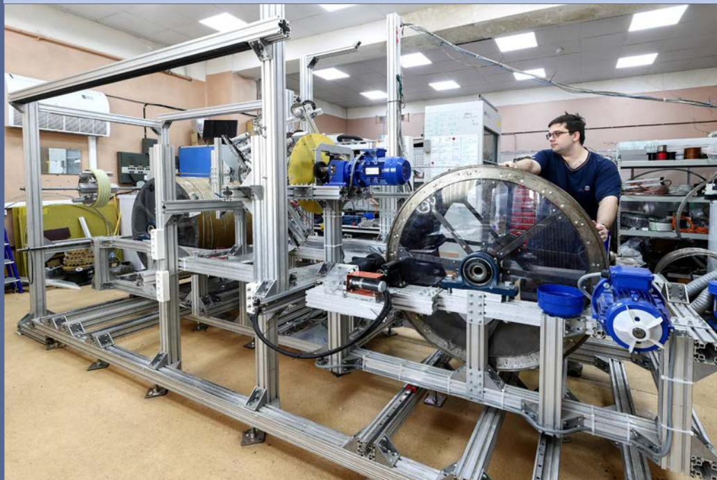
Installation of the HTS magnets winding. Preventive inspection of the base for the magnet
