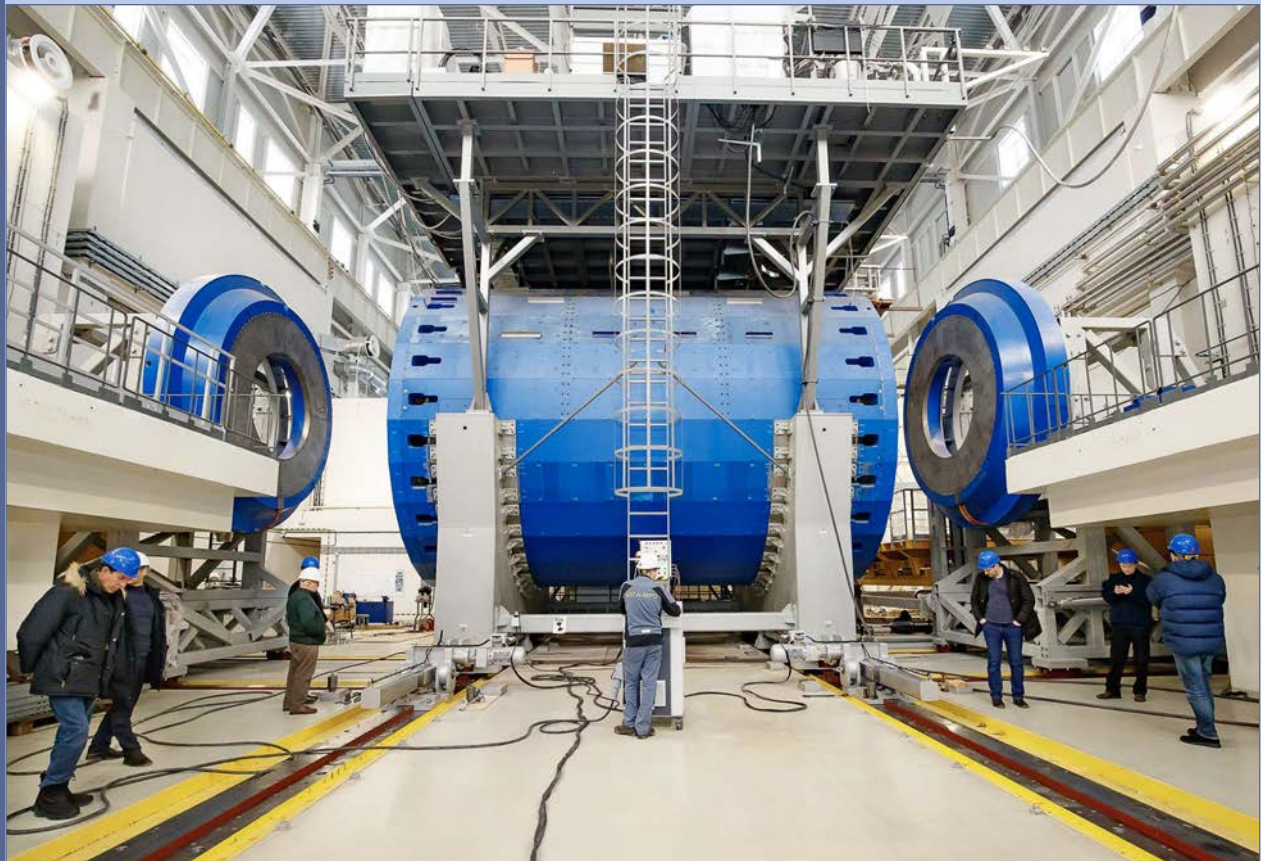
5–6 December. A technological transfer of the 800-ton MPD experiment solenoid in the pavilion of the multipurpose detector of the NICA accelerator complex
