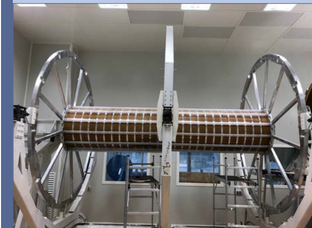
Two flanges and the HV electrode glued with the cylinders C1–C2
